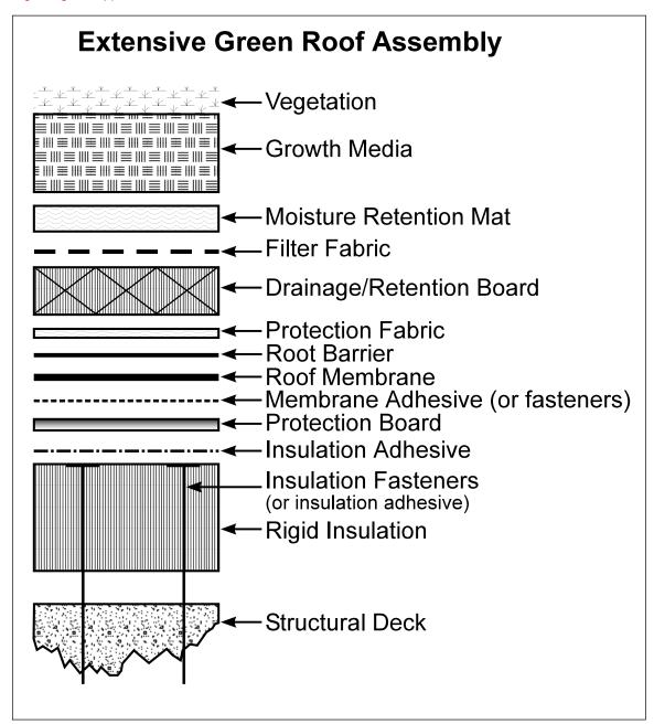
Fig. 1. Sample Extensive green roof assembly
