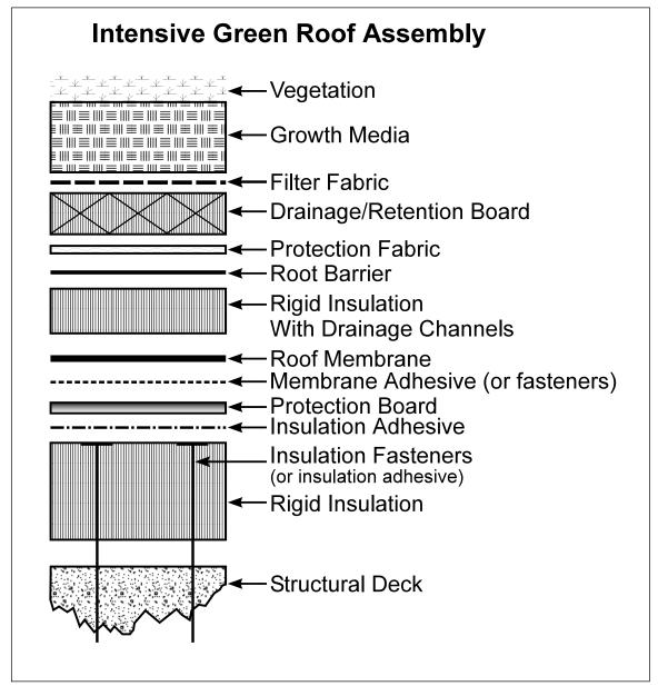
Fig. 2. Sample Intensive green roof assembly
