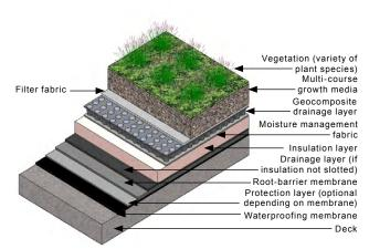
Figure 5: Diagram of a Multi-course Extensive green roof with a PMR configuration
