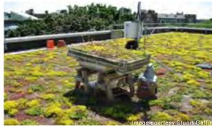
Lysimeter used to measure the amount of evapotransipiration released by plants.
