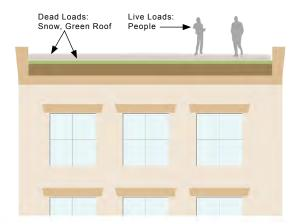
Variations from the design weight can lead to structural failure.
