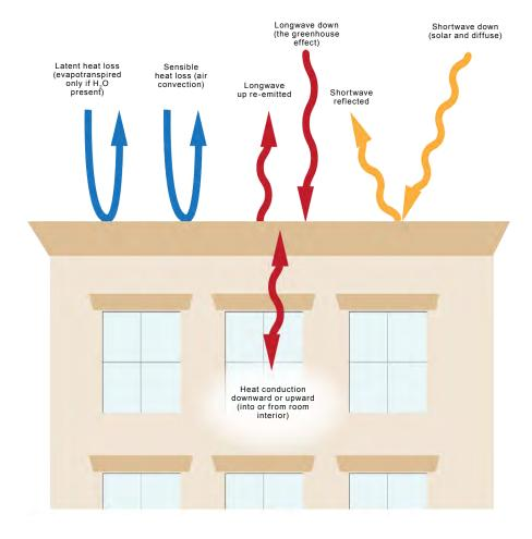
Figure 20: Surface energy balance for a roof
