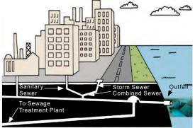
Figure 1: Combined Sewer Overflow network
