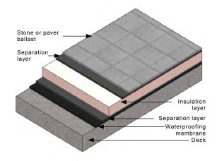
Figure 4: Diagram of a PMR roofing system
