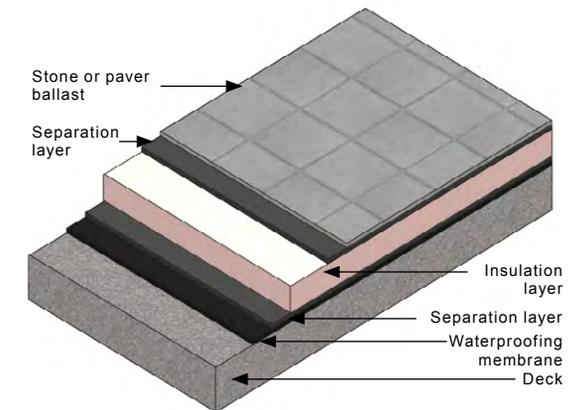
Figure 4: Diagram of a PMR roofing system
