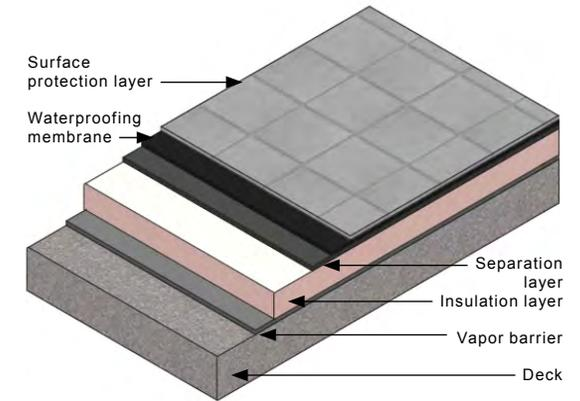
Figure 3: Diagram of a conventional roofing system
