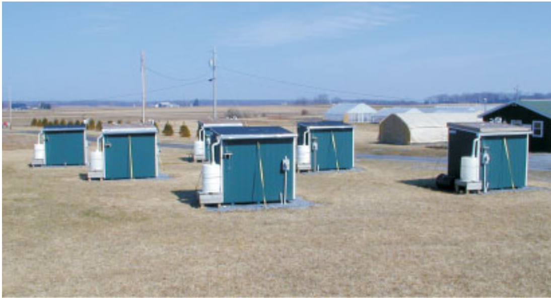
Figure 2. Green and control roof field experiment at Penn State University (9).
