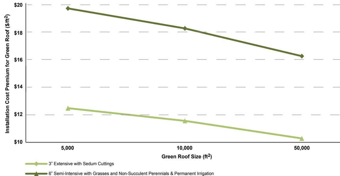
Figure 21: Green roof installation premiums
