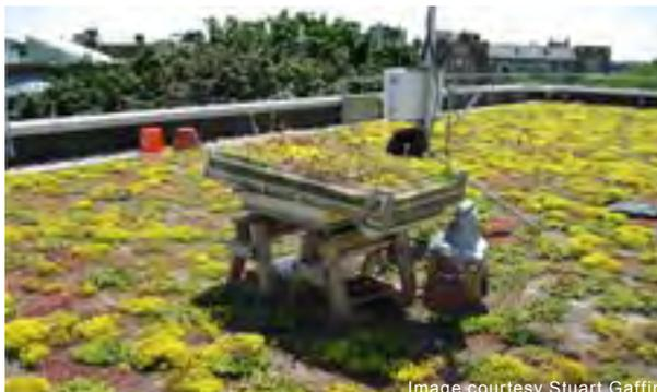
*Lysimeter used to measure the amount of evapotranspiration released by plants.*
